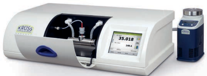
P8000-T with measurement tube PRG-100-ET, temperature probe PRT-T and circulating thermostat PT31
