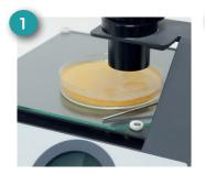
Place the Petri Dish in the Haloes Caliper's **illuminated field**
