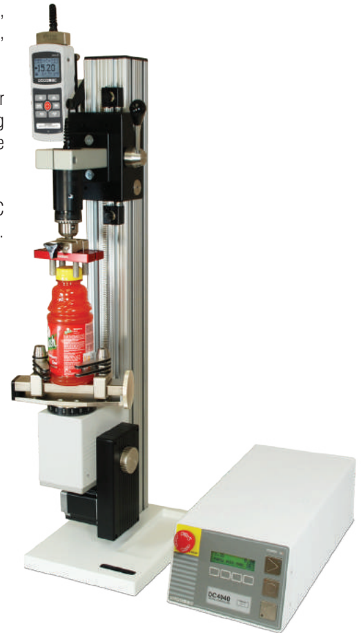
^ Model TSTM-DC is shown in a cap torque test, with a Series R50 torque sensor, M5i force/torque indicator, G1023 universal closure grip, and G1053 cap grip
