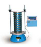
for 200, 250, 300 & 315mm, 8 & 12 inch diameter sieves to EN 932-5, ISO 3310-1 test
