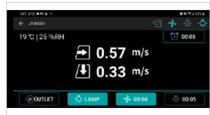
No need to take out hands during the experiment to manipulate controller through Bluetooth, preventing cross-contamination (Option)
