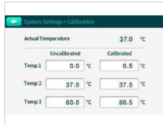
Accurate temperature control with 3-point calibration
