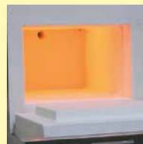
Muffle heated from four sides
