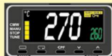
Example of an over-temperature limiter
