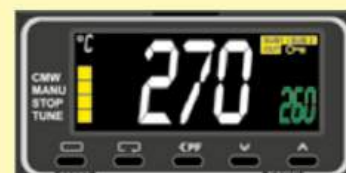
Example of an over-temperature limiter
