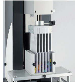
TX-KFBF : KRAMER 5 BLADES FIXTURE (Ref. 130094R) Hardness and tenderness on small samples (Requires table TX-FBT).
