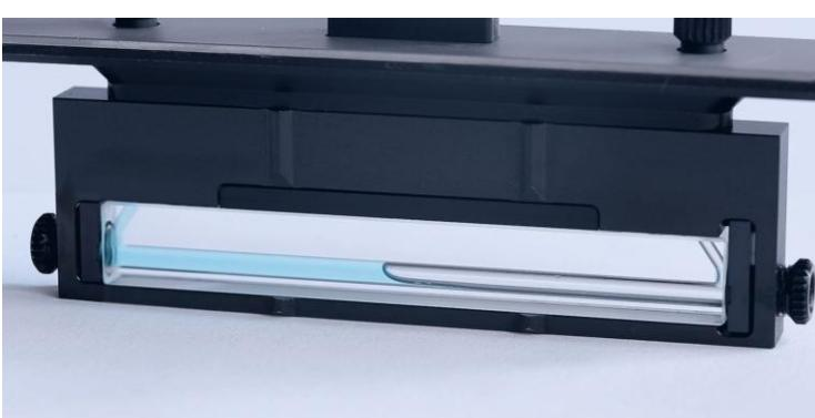
The rectangular shape of our glass cuvettes allows visual control of the sample filling over the entire length of the cuvette.
