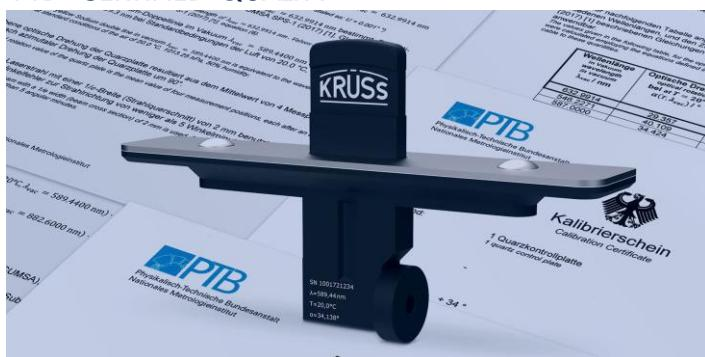
We only use quartz control plates certified by the Physikalisch-Technische Bundesanstalt (PTB) – both for the manufacturer's calibration of our polarimeters and for later use in your laboratory.
