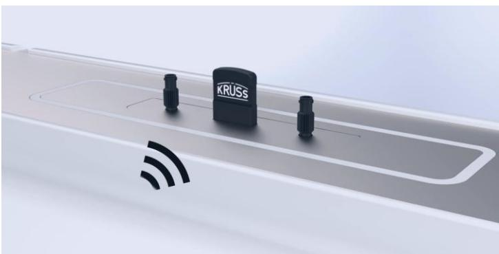
For an intuitive measurement and calibration process, the polarimeter automatically recognizes the cuvette equipped with an RFID tag and records all relevant cuvette data such as:
